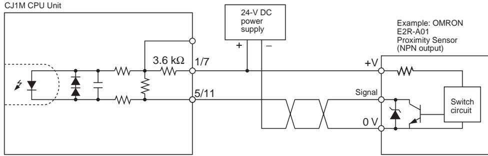
**Origin Input Signal (Line Driver Input)**
