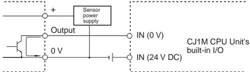
• Device with NPN current output
