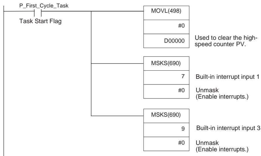
**Built-in Input 1 Interrupt Task (Interrupt Task 141)**
