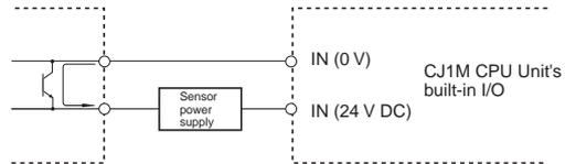
• Device with NPN open collector output
