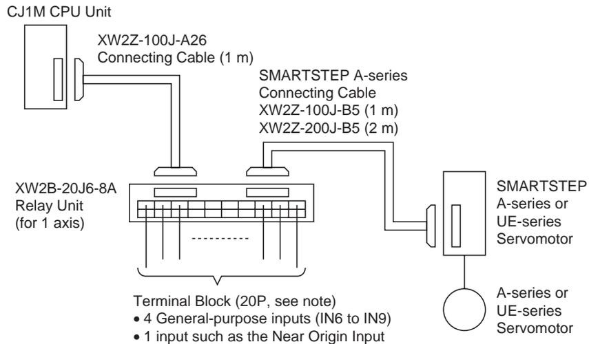
**Note** When using a One-axis Relay Unit (connected to pulse output 0), general-purpose outputs 2 and 3 (OUT2 and OUT3) and PWM(891) output 1 (OUT5) cannot be used.
