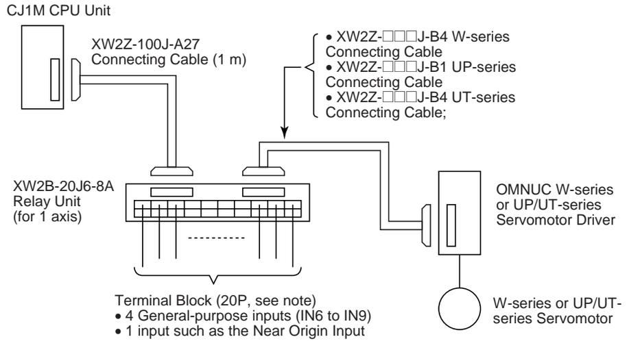
**Note** When using a One-axis Relay Unit (connected to pulse output 0), general-purpose outputs 2 and 3 (OUT2 and OUT3) and PWM(891) output 1 (OUT5) cannot be used.
