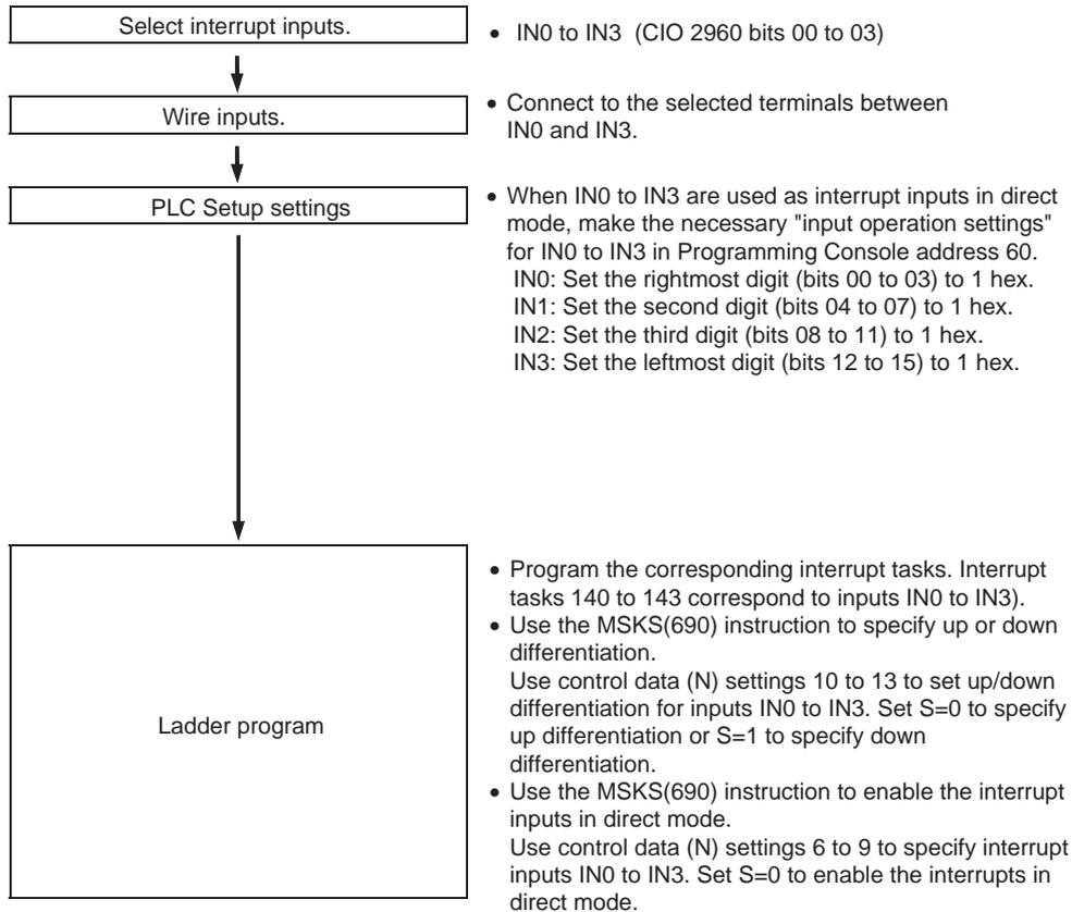
**Note** Use the MSKS(690) instruction to select the interrupt mode (direct mode or counter mode.)
