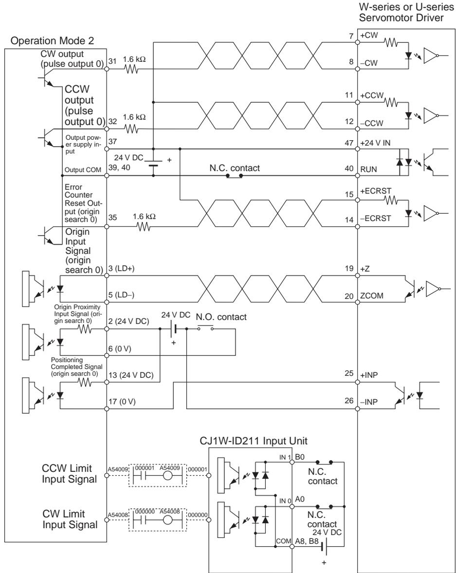
Connecting an OMRON U-series (UE) or SMART STEP A-series Servo Driver
