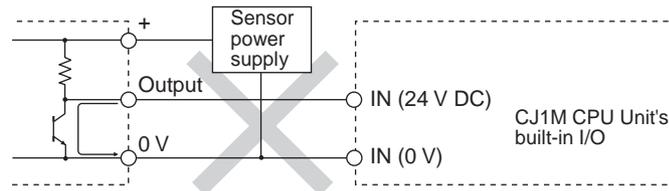
**Note** The CJ1M CPU Unit's inputs have a set polarity, so the inputs will not go ON if the wiring is reversed. Always double-check the wiring before turning ON the power.
