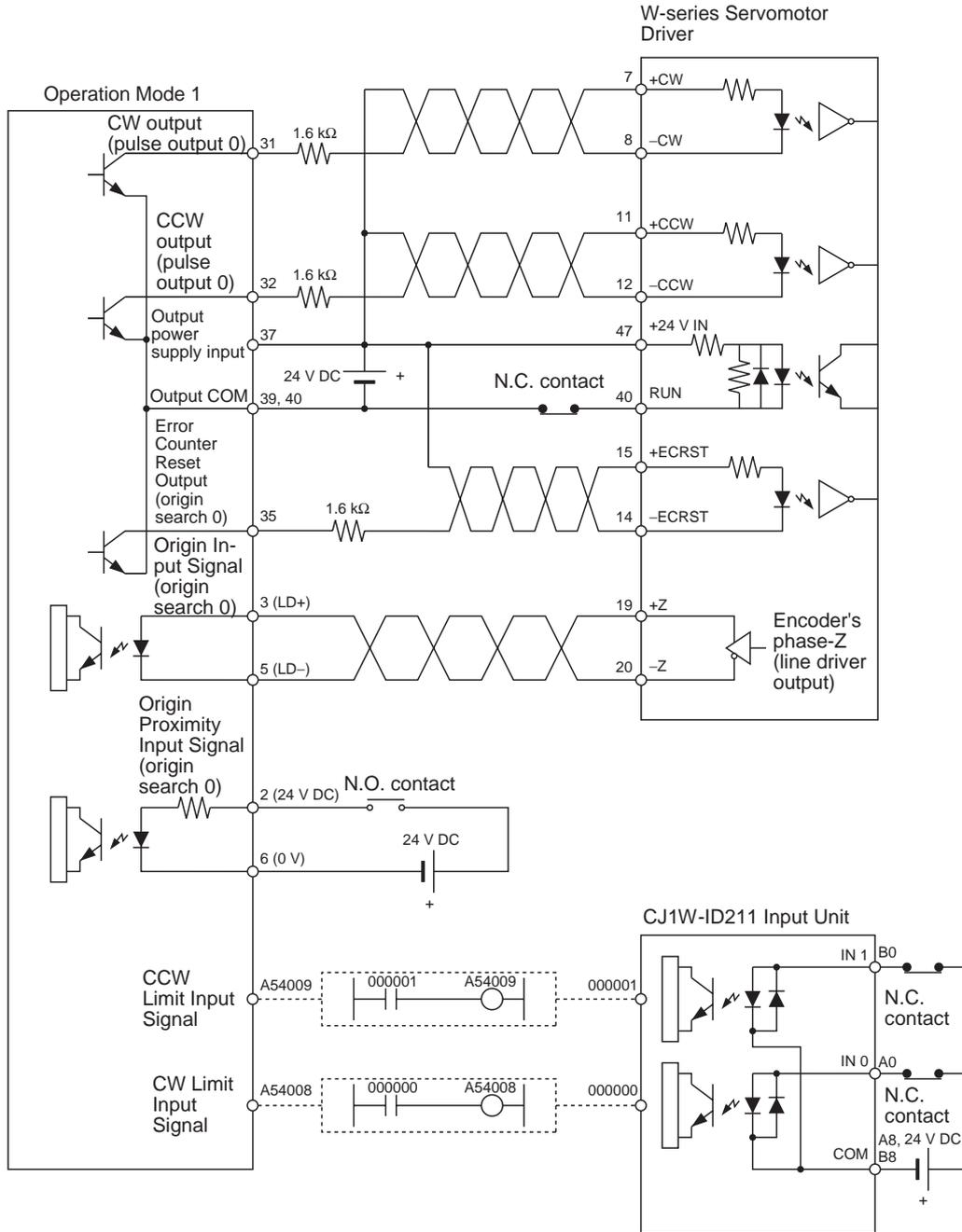
Connecting a SMARTSTEP A-series Servo Driver
