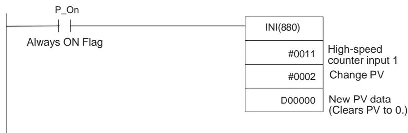
**Built-in Input 3 Interrupt Task (Interrupt Task 143)**
