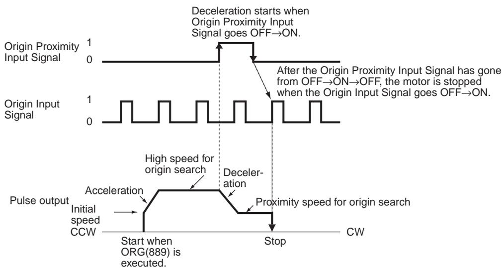
**Origin Detection Method 1: Origin Proximity Input Signal Reversal Not Required**
