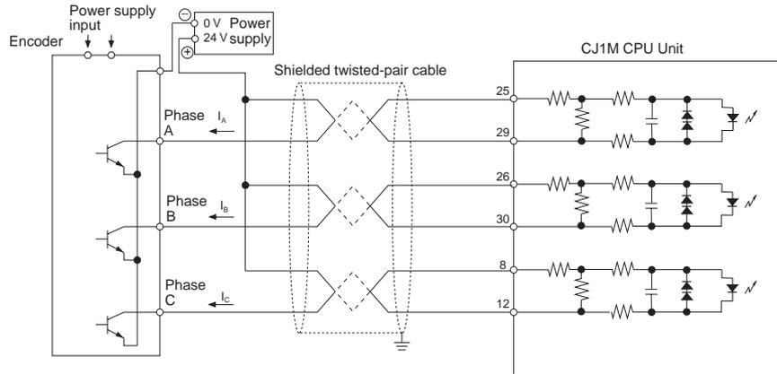
Encoders with Line Driver Outputs (Conforming to Am26LS31)
