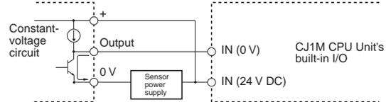
Output; Sensor power supply; IN (0 V); IN (24 V DC); CJ1M CPU Units built-in I/O;
