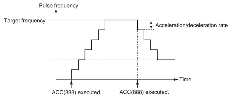
In independent mode, pulse output stops automatically when the specified number of pulses has been output. In continuous mode, pulse output continues until it is stopped from the program.
