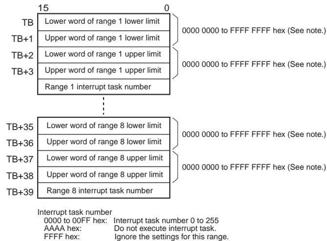
**Note** Always set the upper limit greater than or equal to the lower limit for any one range.
