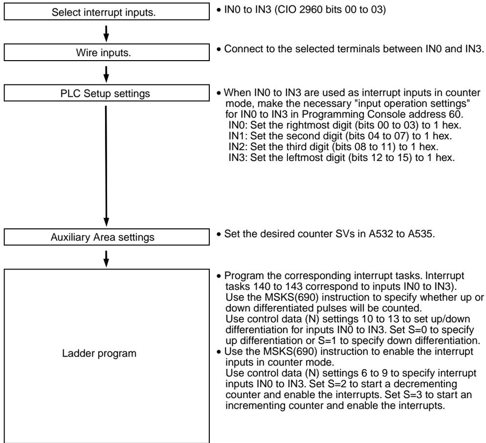
**Note** Use the MSKS(690) instruction to select the interrupt mode (direct mode or counter mode.)
