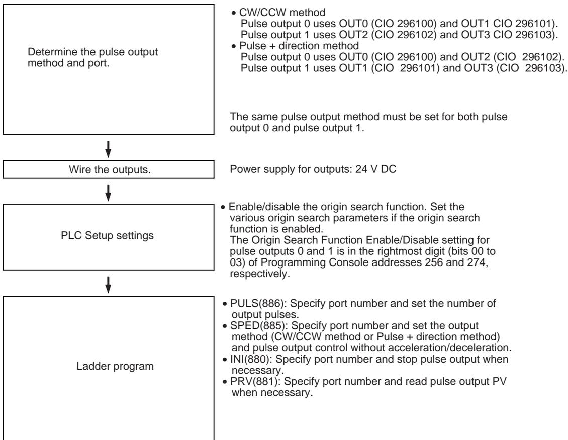
Single-phase Pulse Output with Acceleration/Deceleration
