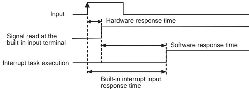
Built-in interrupt input response time = Hardware interrupt response time + Software interrupt response time
