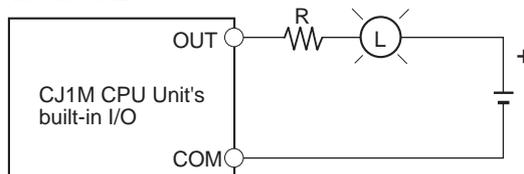
This method uses a limiting resistor.
