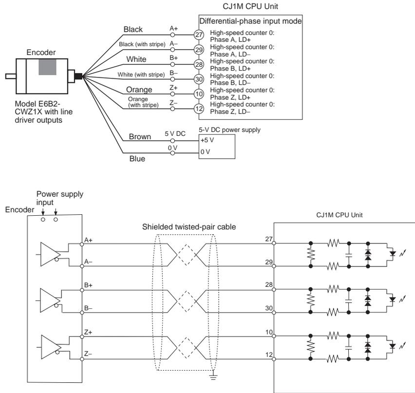
3-3-3 Power Supply Input Connection Example
