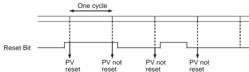
**Note** With CJ1M CPU Unit Ver. 2.0, the comparison operation can be set to stop or continue when a high-speed counter is reset. This enables applications where the comparison operation can be restarted from a counter PV of 0 when the counter is reset.
