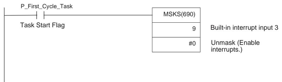
**Built-in Input 3 Interrupt Task (Interrupt Task 143)**
