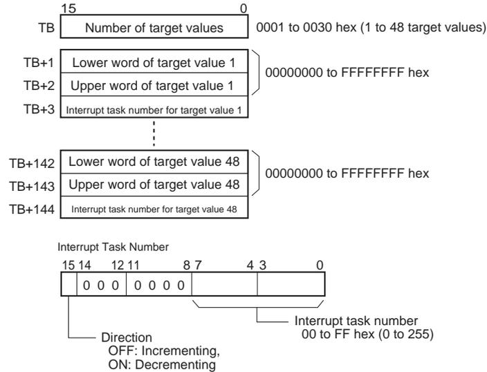
For range comparison, the comparison table always contains eight ranges. The table is 40 words long, as shown below. If it is not necessary to set eight ranges, set the interrupt task number to FFFF hex for all unused ranges.
