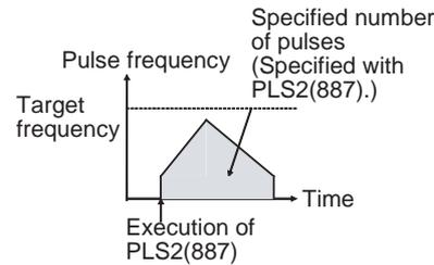
**■ Switching from Continuous Mode Speed Control to Independent Mode Positioning**
