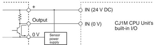
**Note** Do not use the following wiring with voltage-output devices.
