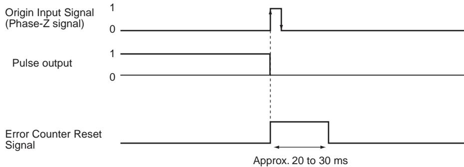
When the Origin Proximity Input Signal is received, the motor will begin decelerating from the origin search high speed to the origin search proximity speed. In this operating mode, the Origin Input Signal will be ignored if it is received during this deceleration. After deceleration is completed, the Origin Input Signal will be detected and the motor will stop.
