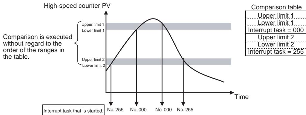
**Note** The range comparison table can be used without starting an interrupt task when the comparison condition is met. The range comparison function can be useful when you just want to know whether or not the high-speed counter PV is within a particular range.
