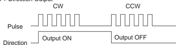
**CW/CCW Pulse Output and Pulse plus Direction Output**
