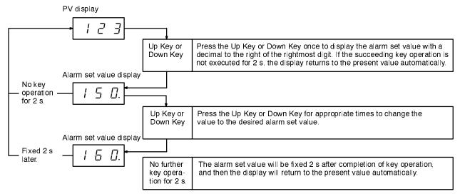
If you change the temperature range after you set the alarm set value, the new alarm set value will remain unchanged. If you change the display unit, the alarm set value will not be converted from the ° C to ° F value or vice versa.
