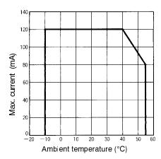
Note: The derating curve shown is for standard installation.
