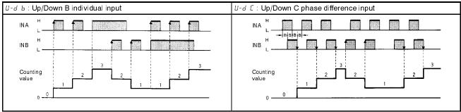
Note: 1. "B" must be larger than half the minimum signal width. If it is smaller, an error of ±1 count may occur.
