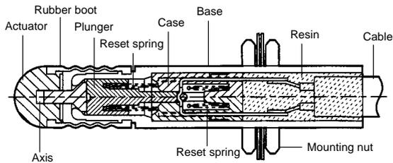
**Note:** NBR rubber is used with this Switch.
