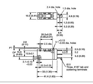
Pin plunger D2VW-01-1MS D2VW-5-1MS
