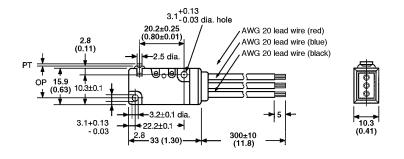
Short hinge lever D2VW-01L1A-1MS D2VW-5L1A-1MS
