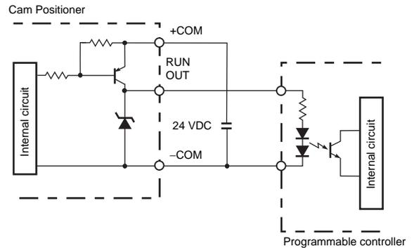
Note: Supply the power to the sensor for INHIBIT signal input and output circuit from the same power source.
