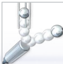
The Ball Drop Test is part of the ATEX approval ensuring high mechanical protection of electronic parts.
