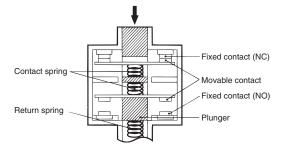
Note: Conforms to EN60947-5-1 Direct Opening. (Only the NC contacts have a direct opening function). When metal weld occurs, the NC contacts are separated from each other by pushing in the plunger.
