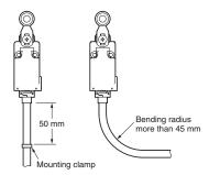
Note: When wiring, be sure to prevent penetration of a liquid such as water or oil through the cable end.
