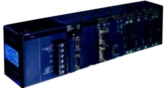
The CJ1 modules are each roughly the size of a deck of playing cards and connect module-to-module using simple locking connectors, eliminating the need for a bulky PLC rack. The lightning quick PC21 bus, designed for Omron's technology-leading mid-sized CS1, provides high-speed communication from the CJ1 CPU to individual modules.
