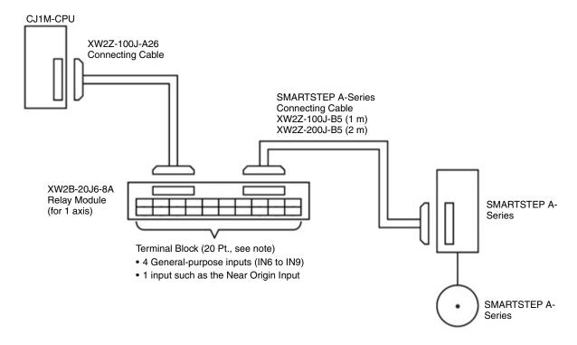
Note: When using a One-axis Relay Module (connected to pulse output 0), general-purpose outputs 2 and 3 (OUT2 and OUT3) and PWM (891) output 1 (OUT5) cannot be used.
