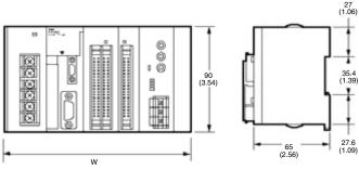
Note "W" is determined by total width of power supply, CPU, I/O Modules and end plate.
