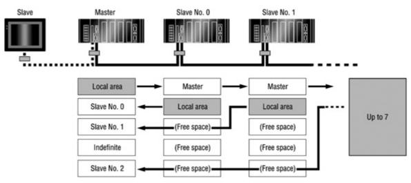
**Note:** An NT/NS-series PT can also be connected as a slave (1:N NT Link). In this case data can be exchanged via NT Link with the master only. It is allocated one slave node.
