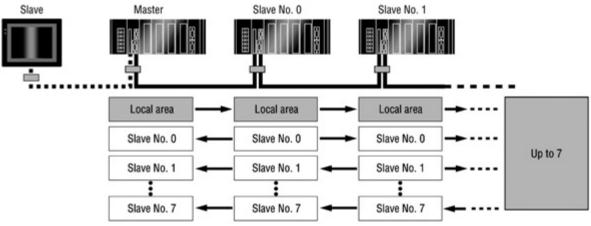
**Note:** An NT/NS-series PT can also be connected as a slave (1:N NT Link). In this case, data can be exchanged via NT Link with the master only. It is allocated one slave node.
