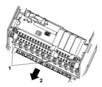
Fig 8.6 Removing the Control Circuit Terminal Card
