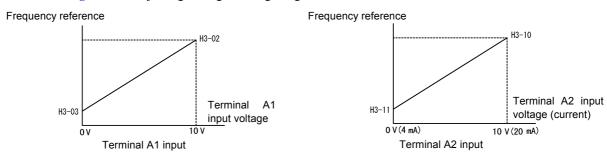
Fig 6.29 Terminals A1 and A2 Inputs
