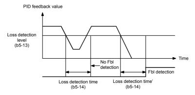
Fig 6.78 Low PID Feedback Loss Detection Time Chart
