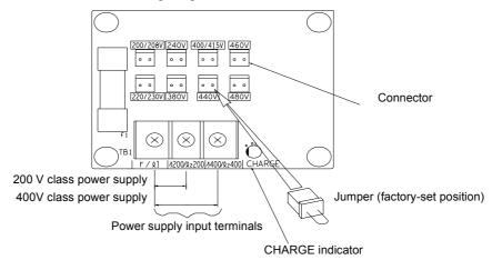
Fig 4.2 Large-capacity Inverter Connections
