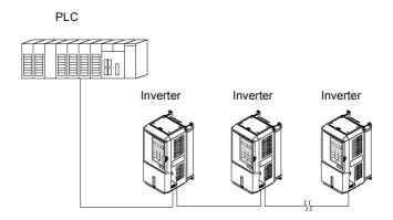
Fig 6.71 Example of Connections between PLC and Inverter
