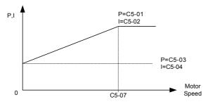
Fig 6.41 Low-speed and High-speed Gain Settings
