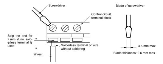
Fig 2.11 Connecting Wires to Terminal Block
