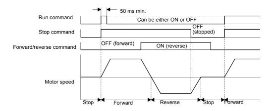
Fig 6.14 Three-wire Control Timing Chart
