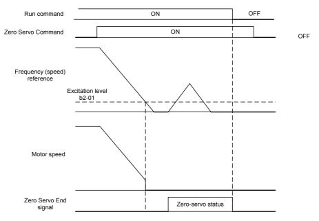
Fig 6.86 Time Chart for the Zero-Servo Function
