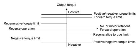
Fig 6.46 Torque Limits using the Analog Input
