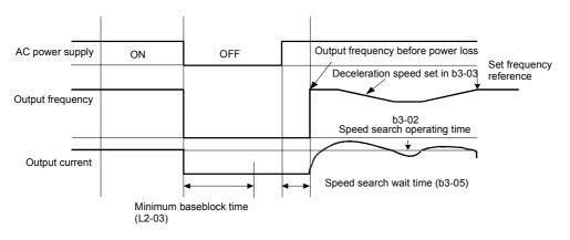
Fig 6.60 Speed Search after Power Loss with Loss Time > L2-03
