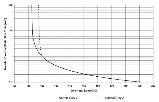
Fig 6.4 Normal Duty 1 and 2 Inverter Overload Detection Curve
