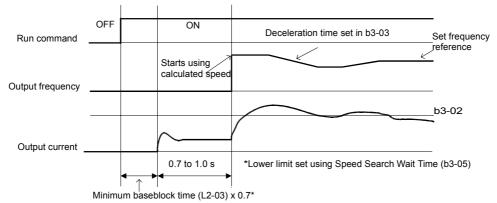
Note: If the stopping method is set to coast to stop, and the run command turns ON in a short time, the operation may be the same as the search in case 2.
