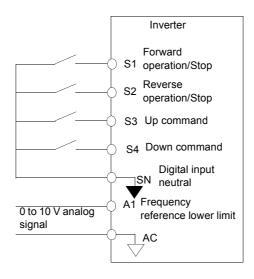
Fig 6.65 Connection Example when UP/DOWN Commands Are Allocated
