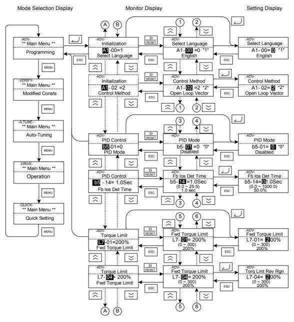
Fig 3.6 Operations in Advanced Programming Mode
