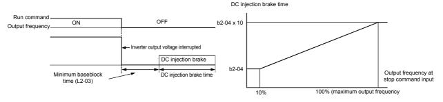
Fig 6.18 DC Injection Braking to Stop
