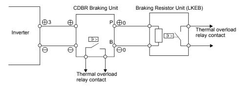
Fig 2.8 Connecting the Braking Resistor and Braking Unit
