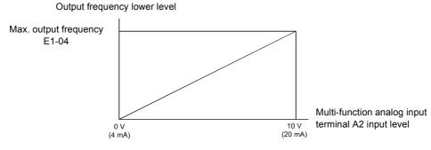
Fig 6.35 Analog Input A2 Charecteristics for Frequency Reference Lower Limit
