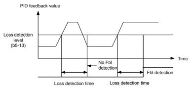
Fig 6.79 High PID Feedback Loss Detection Time Chart
