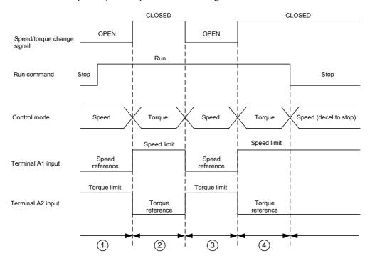
Fig 6.84 Speed/Torque Control Switching Time Chart
