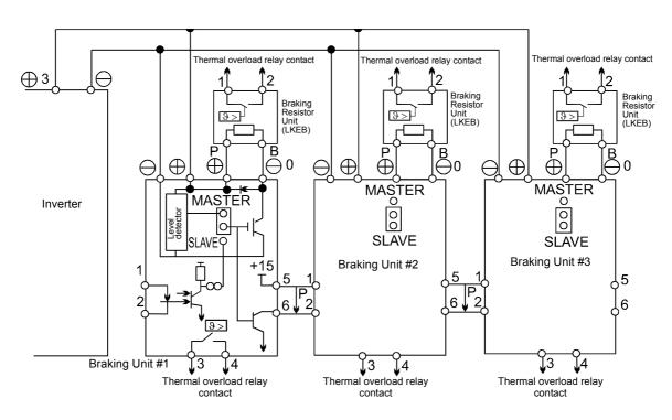
Fig 2.9 Connecting Braking Units in Parallel
