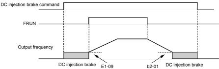
If you input the DC injection brake command from an external terminal, and if a run command or jog command is input, the DC injection brake will be disabled, and operation will resume.
