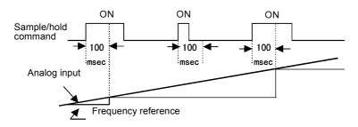
Fig 6.67 Sample/Hold Analog Frequency
