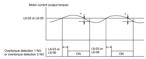
\*Overtorque detection switch off bandwidth is approximately 10% of the Inverter rated output current (or motor rated torque).
