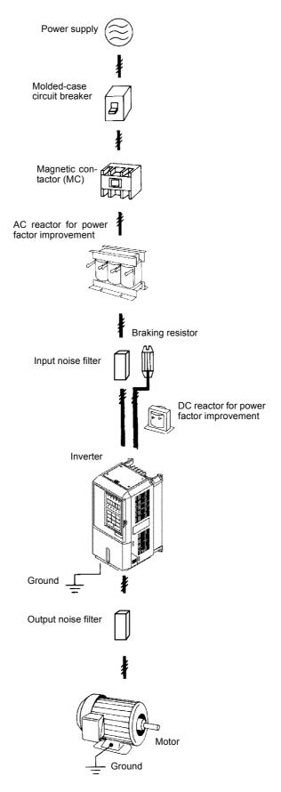
Fig 2.1 Example Connections to Peripheral Devices
