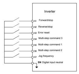
Fig 6.10 Control Circuit Configuation for 9-step Operation
