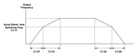
When output frequency  $\geq$  C1-11, acceleration and deceleration are performed using Acceleration/deceleration Time 1 (C1-01, C1-02).
