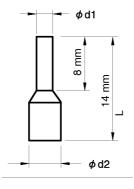
Fig 2.10 Straight Solderless Terminal Sizes
