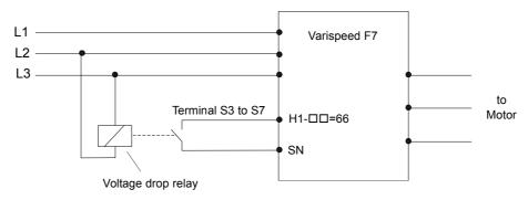
Fig. 6.87 Wiring Example for KEB function usage
