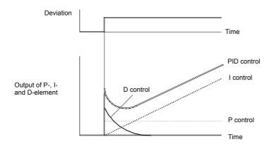
Fig 6.76 PID Control Operation
