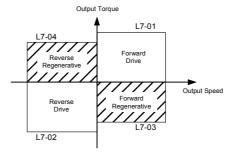
Fig 6.45 Torque Limit Paremeters
