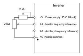
Fig 6.6 Master Speed Frequency Reference Input
