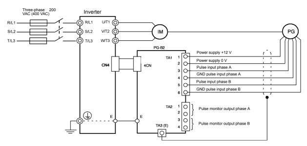
Fig 2.16 PG-B2 Wiring Using the Option Cards Power Supply
