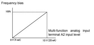
Fig 6.31 Frequency Bias Adjustment (Terminal A2 Input)
