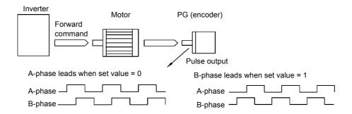
Example: Forward rotation of standard motor (PG)
