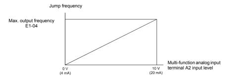
Fig 6.33 Jump Frequency Setting Using an Analog Input
