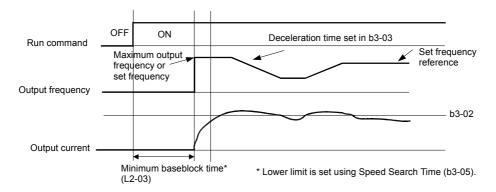
Fig 6.58 Speed Search at Startup (Current Detection)
