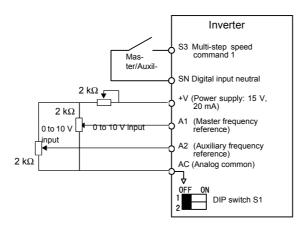
Fig 6.7 Master/Auxiliary Frequency Reference Input
