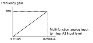
Fig 6.30 Frequency Gain Adjustment (Terminal A2 Input)
