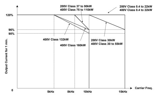
Fig 6.3 Overload Capabilty in Normal Duty 1 Mode
