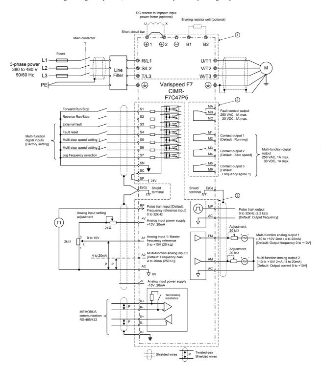
Fig 2.2 Connection Diagram (Model CIMR-F7Z47P5 Shown Above)
