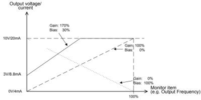
Fig 6.70 Monitor Output Adjustment
