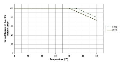
Fig 6.61 Ambient Temperature Derating Curve
