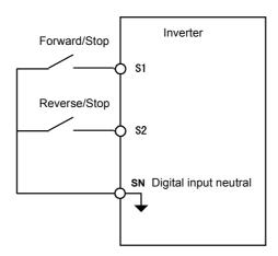
Fig 6.12 2-Wire Control Wiring Example with Positive Logic
