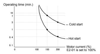
Fig 6.52 Motor Protection Operation Time
