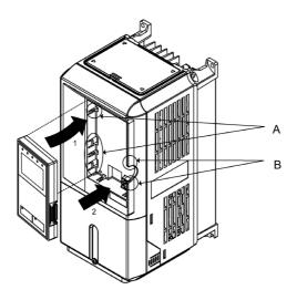
Fig 1.15 Mounting the Digital Operator
