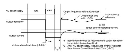
Fig 6.59 Speed Search after Power Loss Time < L2-03
