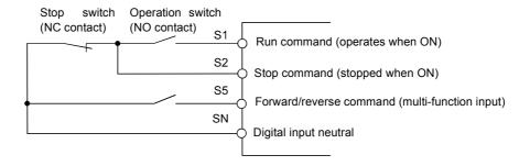
Fig 6.13 3-Wire Control Wiring Example
