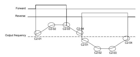
Fig 6.24 S-curve Characteristic during Operation Switching
