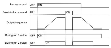
Fig. 6.68 Timing Chart for "During RUN" Output
