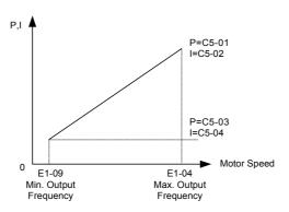
Fig 6.43 Speed Control Gain Integral Time Adjustment for V/f Control with PG
