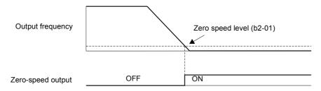
Fig 6.69 Timing Chart for Zero-speed
