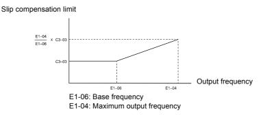
Fig 6.36 Slip Compensation Limit
