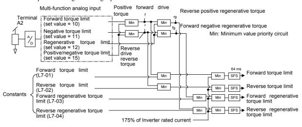
Fig 6.47 Torque Limit Using Parameters and an Analog Input Together
