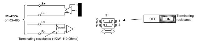
Fig 6.72 Communications Connection Terminal
