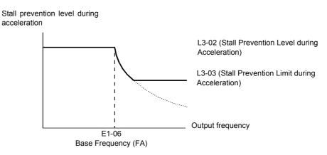
Fig 6.27 Stall Prevention Level and Limit During Acceleration
