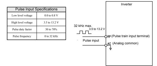
Fig 6.9 Frequency Reference Using Pulse Train Input
