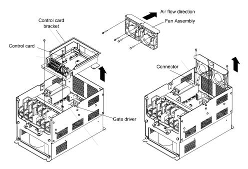
Fig 8.5 Cooling Fan Replacement (Inverters of 22 kW or More)
