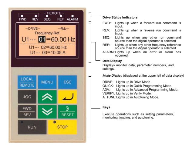
Fig 3.1 Digital Operator Component Names and Functions
