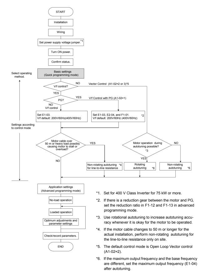
Fig 4.1 Trial Operation Flowchart
