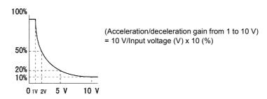
Fig 6.23 Acceleration/Deceleration Time Gain Using an Analog Input
