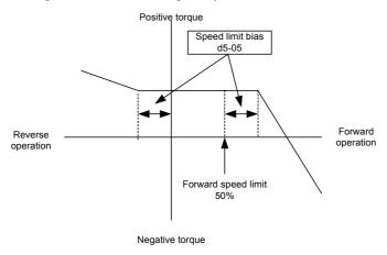
Fig 6.83 Speed Limit Bias Setting
