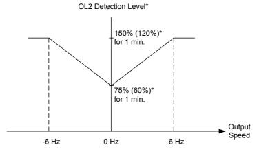
\* Note that the OL2 level depends on the setting of C6-01. The values are given for Heavy Duty. The values in parentheses are for Normal Duty 1 or 2.
