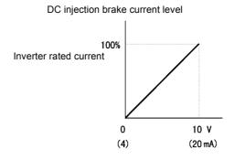
Fig 6.21 DC Injection Brake Current Using an Analog Input
