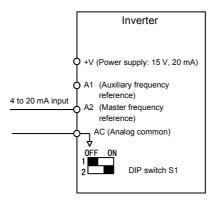
Fig 6.8 Frequency Reference Using Current
