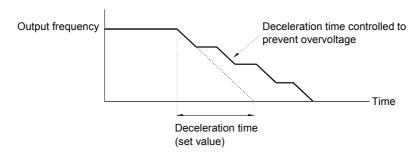
Fig 6.28 Stall Prevention During Deceleration Operation
