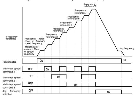
Fig 6.11 Multi-step speed command/Jog Frequency Selection Time Chart
