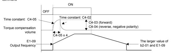
Fig. 6.37 Time Chart for Starting Torque Frequency
