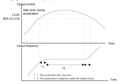
Fig 6.26 Time Chart for Stall Prevention During Acceleration
