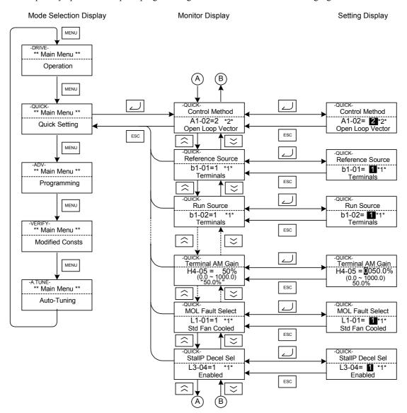
Fig 3.5 Operations in Quick Programming Mode
