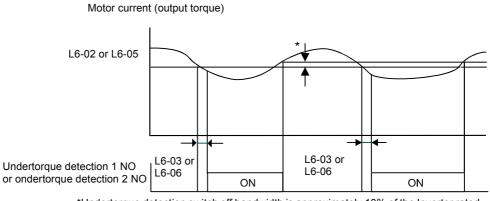
\*Undertorque detection switch off bandwidth is approximately 10% of the Inverter rated output current (or motor rated torque).
