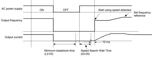
Note: If the frequency immediately before the baseblock is low or the power supply break time is long, operation may be the same as the search in case 1.
