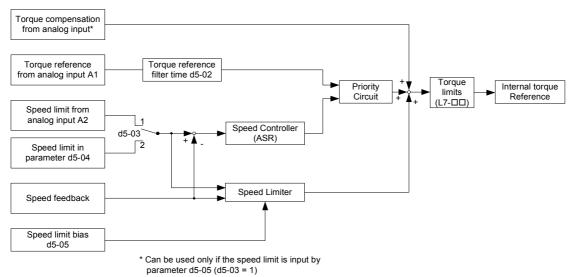
Fig 6.82 Torque Control Block Diagram
