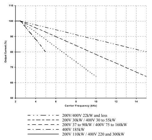
Fig 6.2 Current Derating in Heavy Duty Mode
