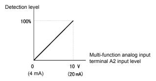
Fig 6.51 Overtorque/Undertorque Detection Level Using an Analog Input
