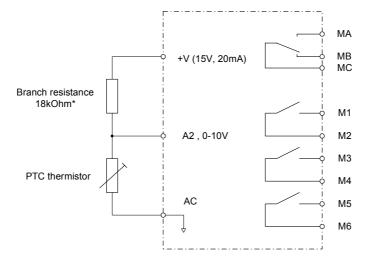
$<sup>^{*1}</sup>$  The resistance value of 18 k $\Omega$  is only valid when a 3-phase PTC with the characteristic shown on the previous page is used.
