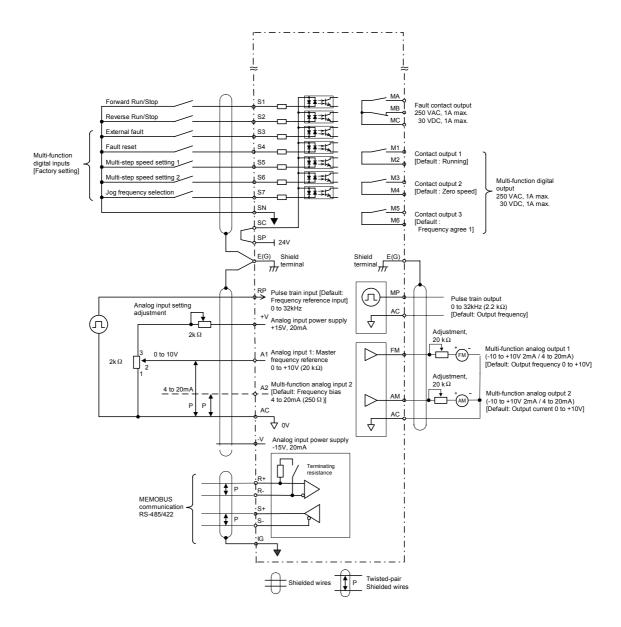
Fig 2.14 Control Circuit Terminal Connections
