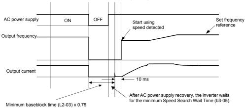
Fig 6.56 Speed Search after Power Loss with Loss Time < L2-03
