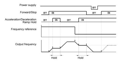
Fig 6.64 Acceleration/Deceleration Ramp Hold
