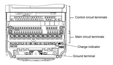
Fig 1.5 Terminal Arrangement (18.5 kW or Less)
