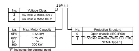
Fig 1.3 Inverter Specifications
